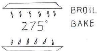
Rather than side by side, perhaps the Broil and Bake indicators should be aligned vertically {see fig. 5}. This could prevent errors in which the operator is mistaken as to the mode of the oven, such as might be created by confusion regarding the meaning of the bake and broil icons.
