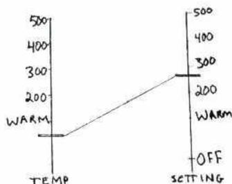
Fig. 4 An alternative display where the slope indicates the direction of temperature change
